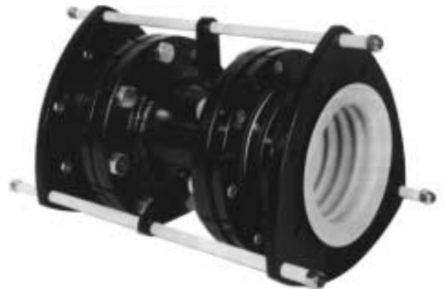
Figure 6 Universal Flexijoint®: Two Flexijoints tied together by a flanged pipe spool in the middle. Gives maximum amount of angular and parallel movement. Substantially reduces the amount of force (spring rate) required to cause movement.
